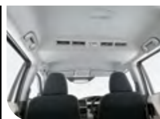
Rear Air Conditioning
